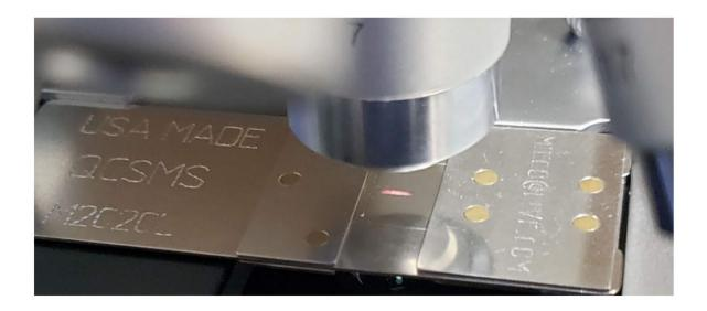
The new M2020L, is a high-quality stainless steel device 2.7'' (68 mm) x 1.0'' (25 mm). Therefore, it fits any sample holder of a microscope stage.
